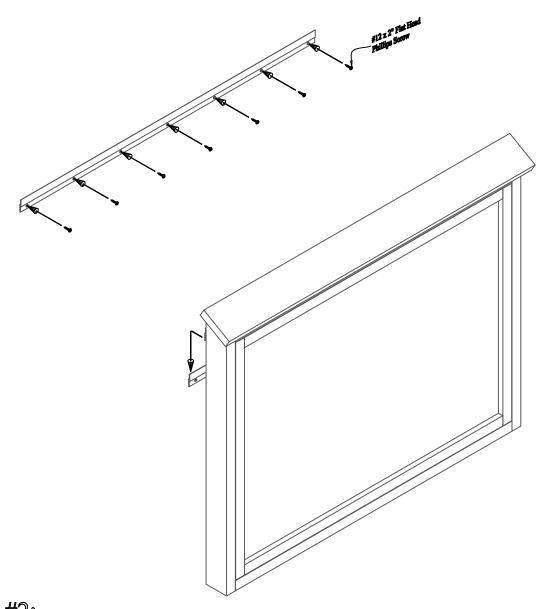
Step #2: Place Message Center above hanger flat against surface then slide down and inter lock the hangers.
