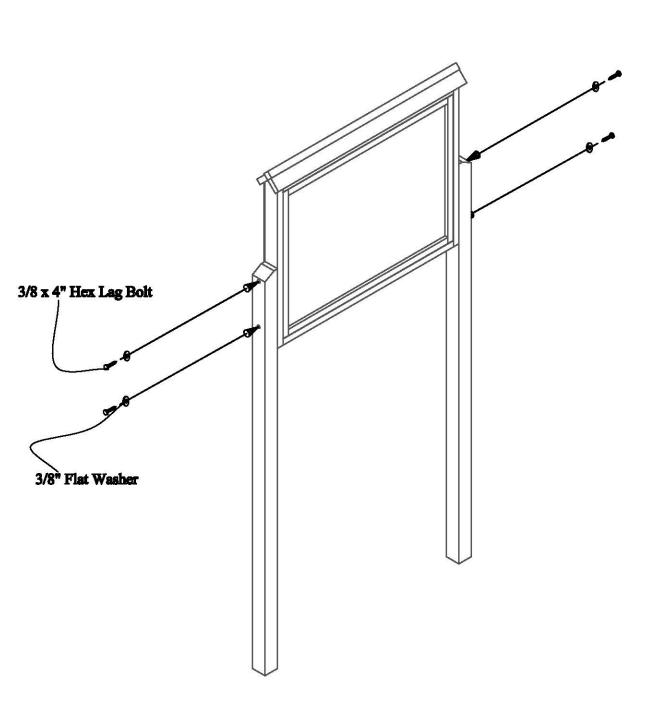
Align the pre drilled holes in the Posts with the pilot holes on the Message center and fasten them together with (1) - one 3/8" Flat Washer & (1) - one 3/8"x 4" Hex Lag Bolt per aligned hole.
