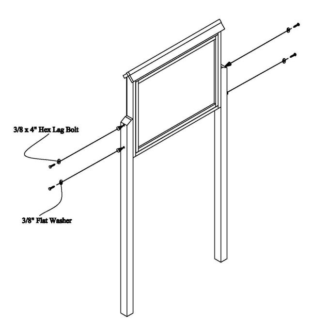
Align the pre drilled holes in the Posts with the pilot holes on the Message center and fasten them together with (1) - one 3/8" Flat Washer & (1) - one 3/8"x 4" Hex Lag Bolt per aligned hole.
